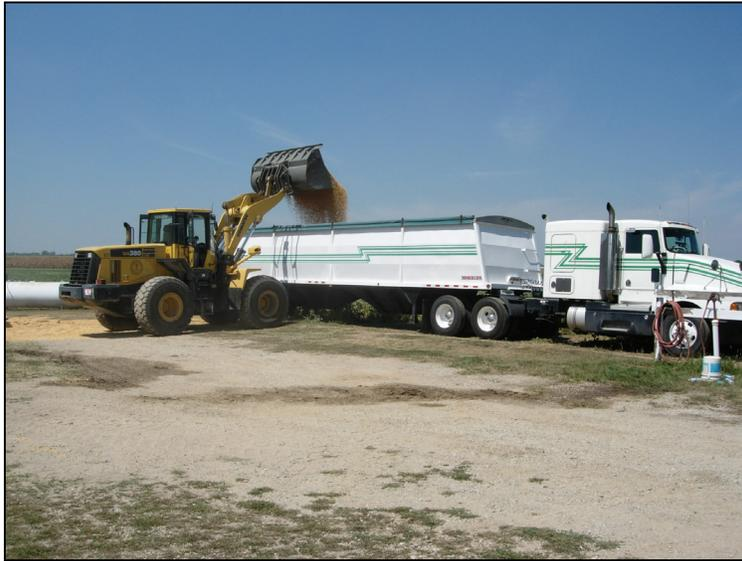
**Figure 5. Front end loader filling a semi-truck trailer during clean-up following the case study extrication.**
