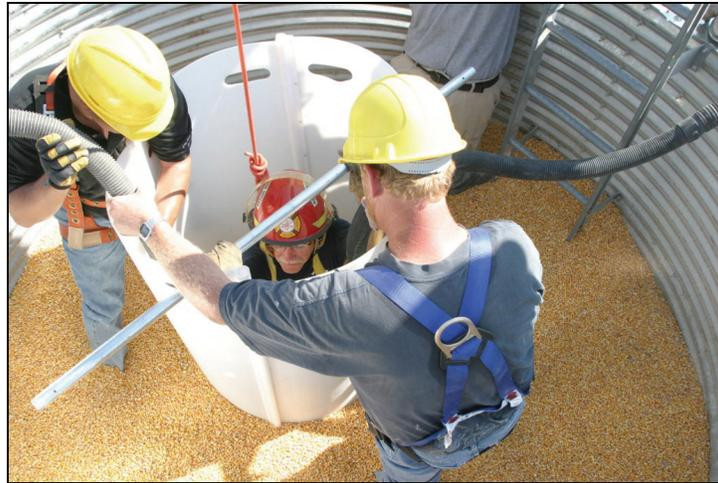
**Figure 2. Commercially manufactured grain rescue tube used in an extrication exercise.**
