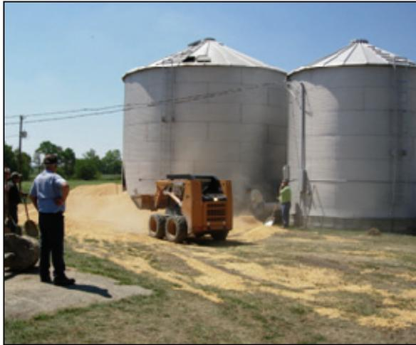
**Figure 6. Skid steer loader removing grain from around the grain bin.**
